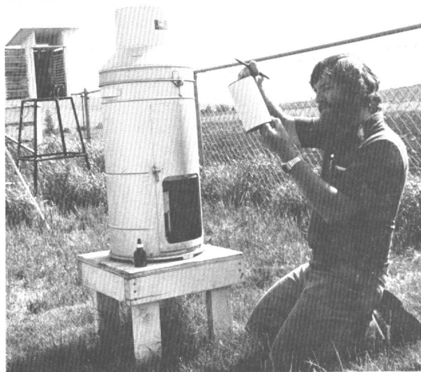
Hydrologic technician removing a raingauge chart at a research site. The automated station is in the background.
