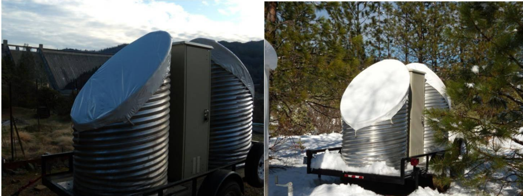
Figure 1. Snow level radar installations at Lake Shasta (left) and Colfax (right).
