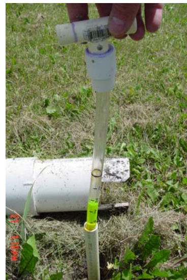
Figure 2. Tygon™ plastic tube filled with water/Orcoacid™ fluoresceine dye mixture
