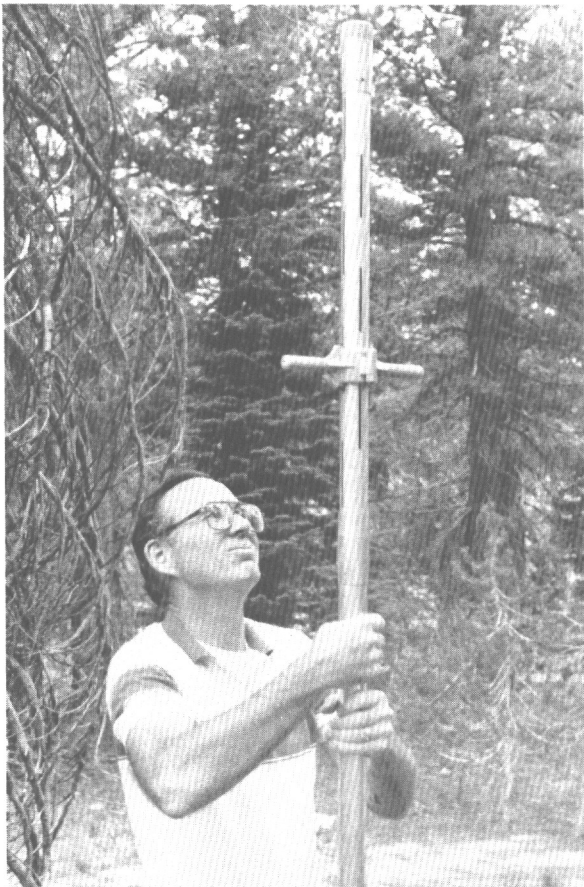
Dr. Donald T. Jensen demonstrates a snow core device used to determine the meltwater equivalent of the snow pack.
